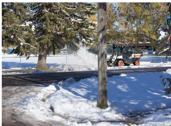
Figure 15 a: Good example of snow removal to support pedestrian travel.
